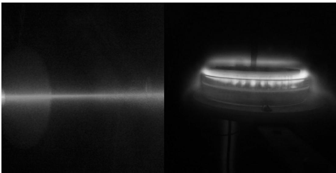
**Fig.2.** Experimental configuration for generation of non-thermal plasmas, on the left real operation of Electron-Beam Plasma, on the right real operation of Radio Frequency Plasma discharge.
