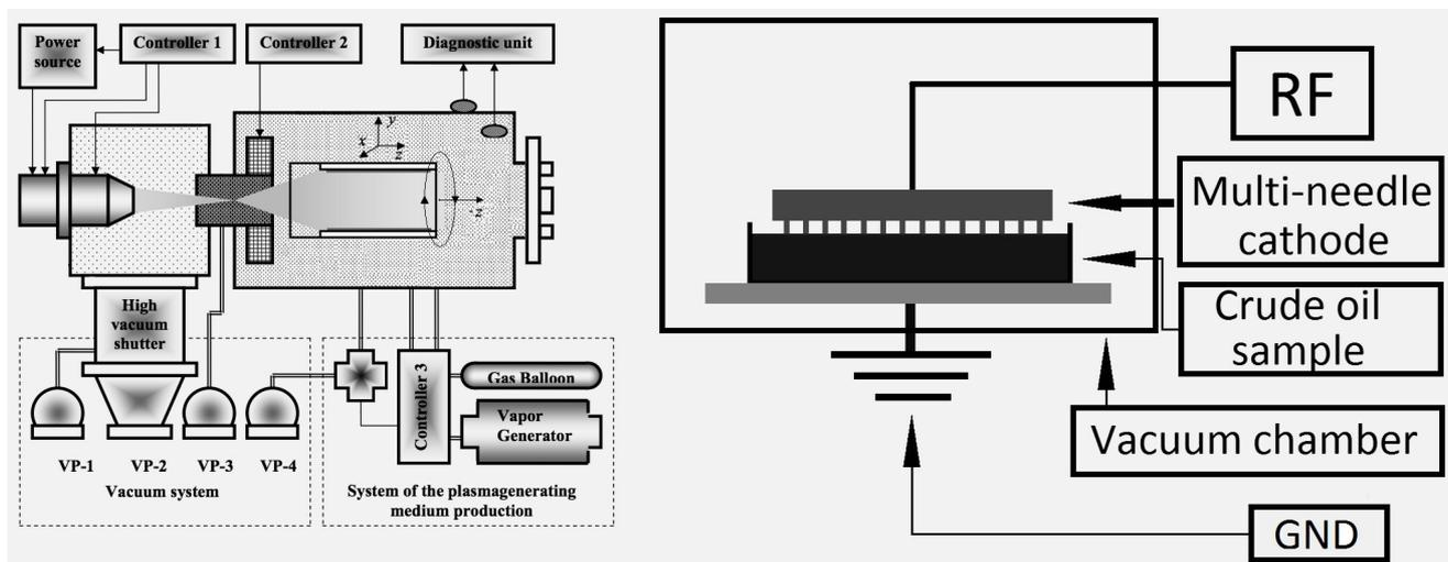
**Fig.1.** Experimental configuration for generation of non-thermal plasmas, on the left configuration for generation of electron-beam plasma, on the right configuration for generation of RF Discharge
