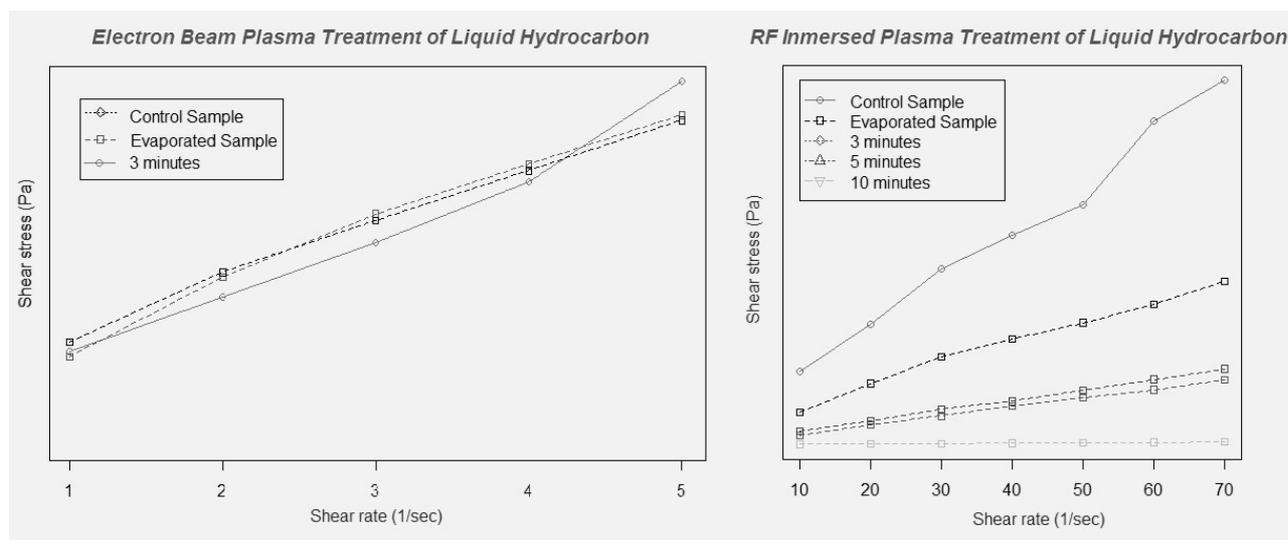
**Fig.3.** Viscosity of the hydrocarbons treated with non-thermal plasma, in the left samples of vacuum oil treated with Electron-Beam Plasma (EBP) and on the right samples treated with RF Plasma discharge.
