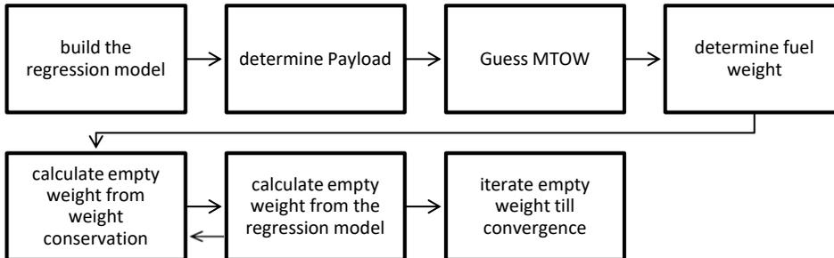
Figure 3. Weight estimation procedure.
