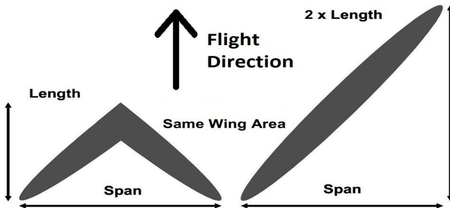
Figure 1. Comparison between swept wing and oblique wing.
